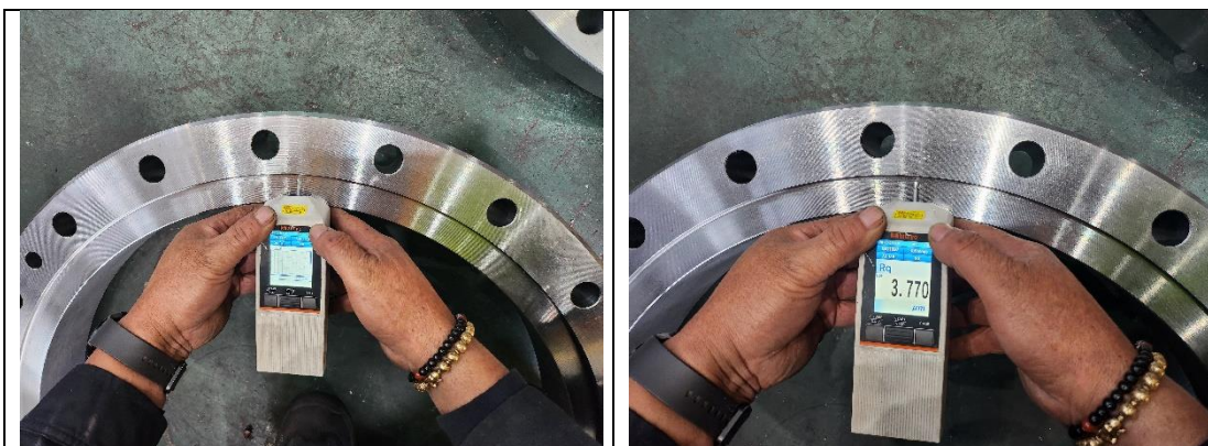
Girth Flange and Test Flange: Visual Dimension, Marking Inspection
