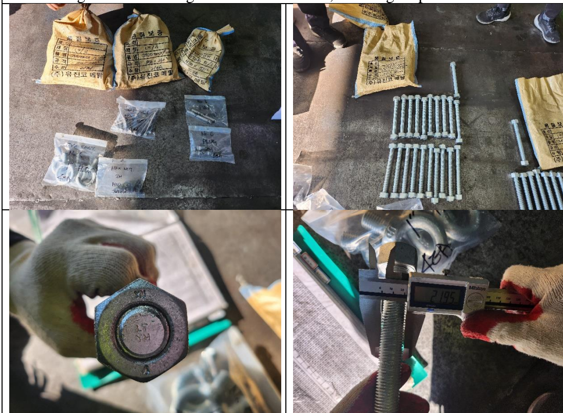
Girth Flange and Test Flange: Visual Dimension, Marking Inspection
